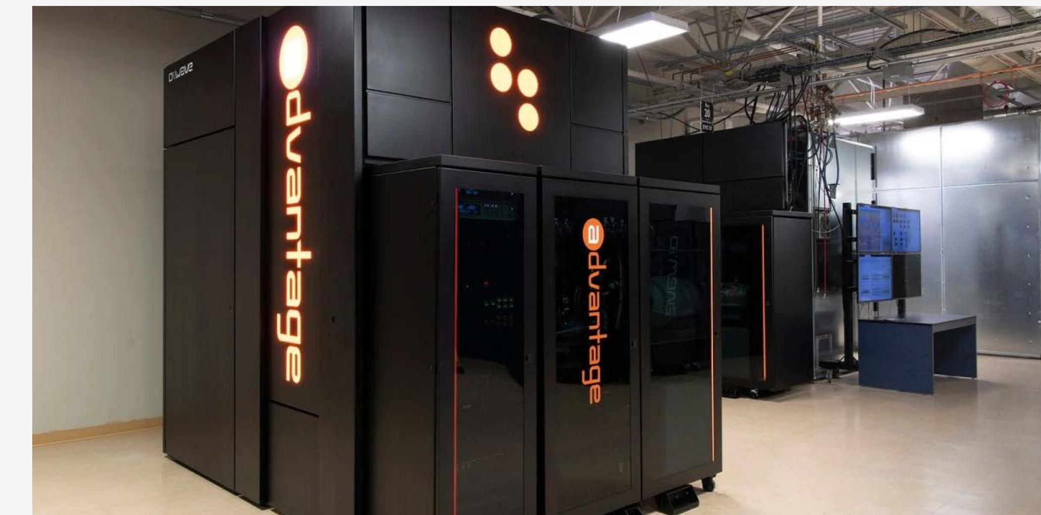
**September 2020** D-Wave – “Advantage contains at least 5,000 qubits, about 2.5 times more than found in a DWave 2000. The number of couplers per qubit has increased from 6 to 15, for a total of at least 35,000 couplers, representing about a six-fold increase over the earlier system.”
